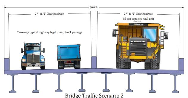
One-way mine haul unit travel with two-way highway truck travel.
